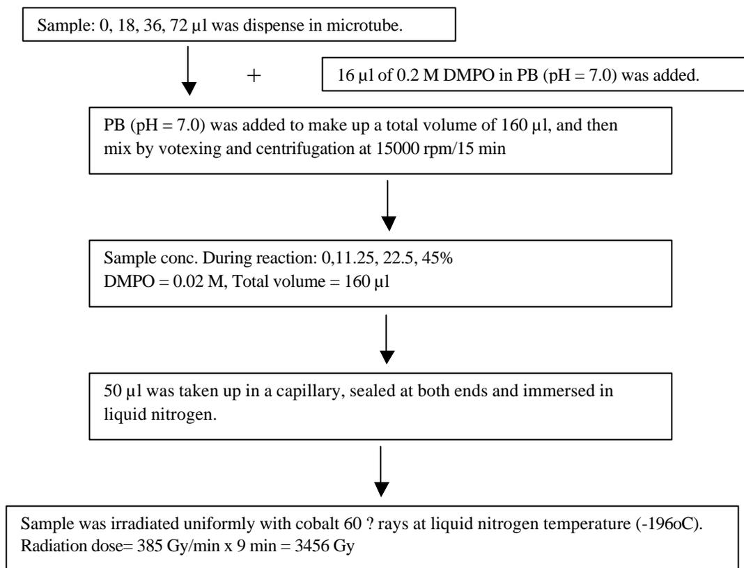
Fig. 2. Hydroxy Radical Eliminating Capability Using ESR
