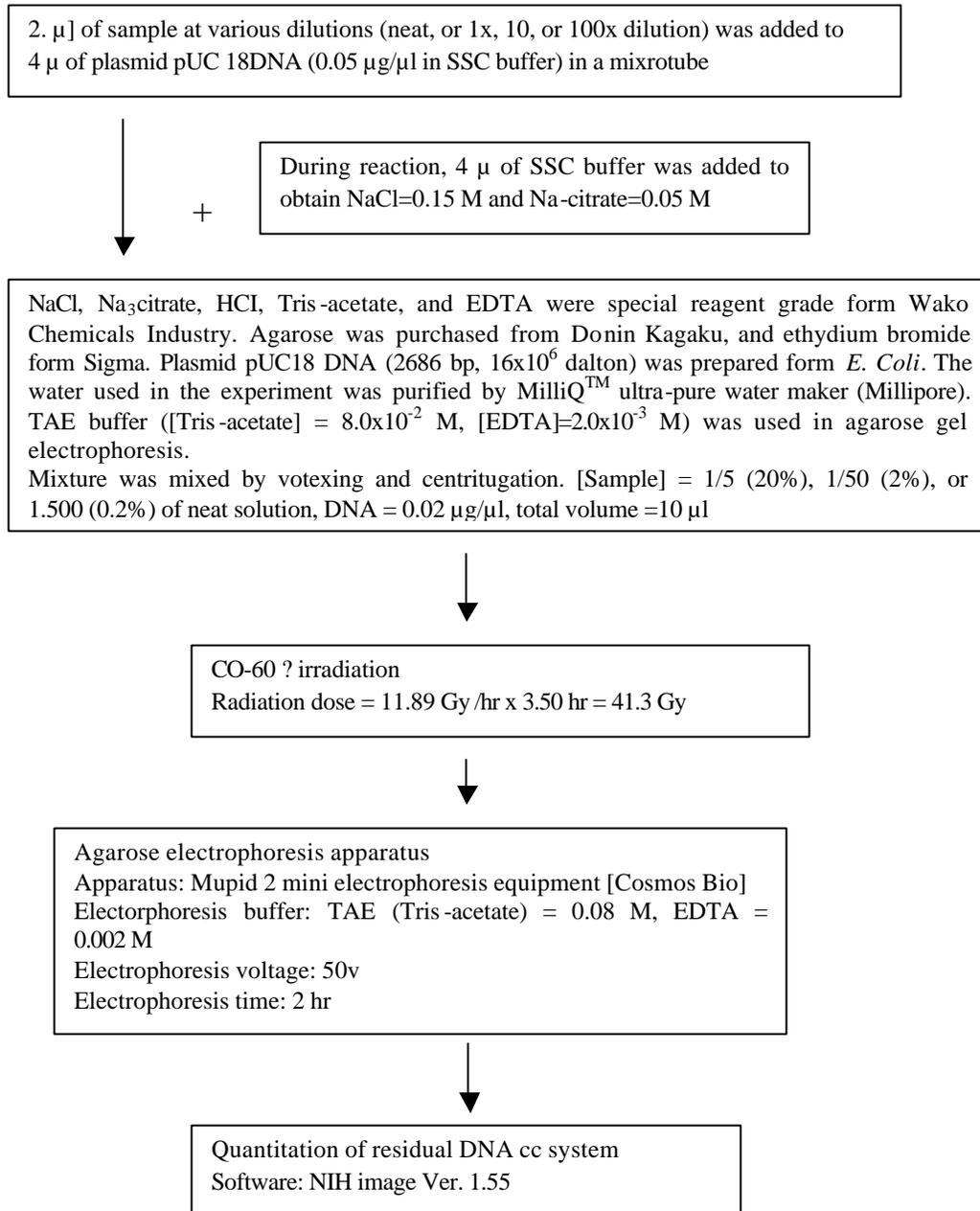
Fig. 1 Methods of Testing Hydroxy Radical Eliminating Capacity Using DNA
